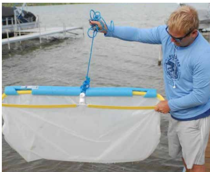
MODIFIED POOL SKIMMER THAT CAN BE DRAGGED THROUGHOUT A SWIM AREA TO REMOVE SWIMMER'S ITCH-CAUSING LARVAE
